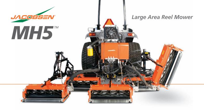
The Jacobsen MH5 tractor-mounted large area reel mower provides a unique, cost-effective alternative to traditional reel mowers. With the ability to mow, verticut or scalp down, the MH5 turns your tractor into a versatile and efficient turf maintenance tool. Achieve excellent ground contour following and productivity with fully floating cutting units and a 135 in. width-of-cut. Each reel is hydraulically driven with enough power and ruggedness to handle even the toughest conditions.
